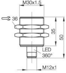
**Inductive Sensors** BES M30MF-GSC15B-S04K M30x1.5 x 50 normally-open Sn=15mm shielded
